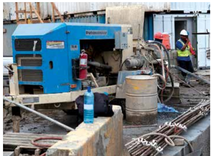
Four Thom-Katt® TK 40 shotcrete machines are at Third Set of Locks, being used to stabilize excavation work on both the Atlantic and Pacific sides of the project.
